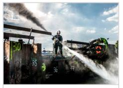
CW1500 Zero Thrust Cavitation Cleaning Gun
